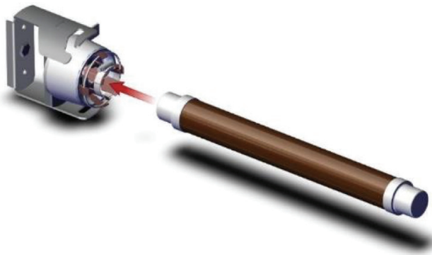
7- Replace the new fuse.
