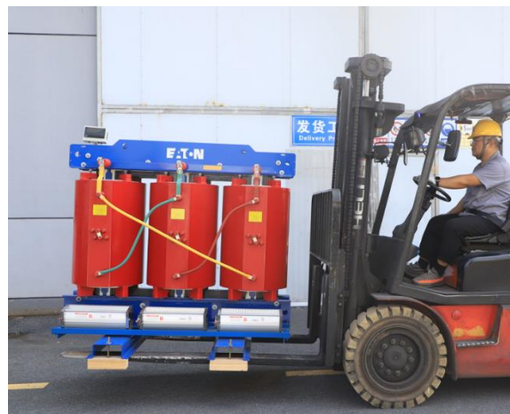
Wooden pallet support packing and fork-lift transportation
